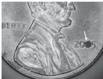
Figure 5.5 Paint fragment placed on the date of a penny for sample size perspective. (See insert for color representation.)
