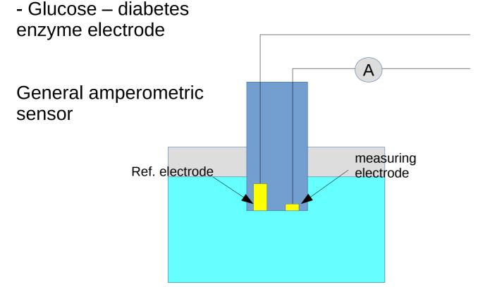
Glucose oxidase reaction can be also used in an amperometric sensor (enzyme electrode). A general amperometric sensor can be composed of measuring and reference electrode. It is immersed into the solution and potential is applied on electrodes. The current is limited by the rate of electrochemical reaction, which is limited by diffusion on the electrode. This process depends linearly on the concentration of the analyte that can react spontaneously on the measuring electrode.
