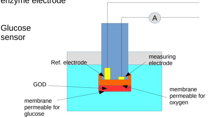
By adding another compartment separated by a membrane permeable only for glucose with glucose oxidase it is possible to measure glucose. These sensors are used in clinical labs or by diabetic patients.
