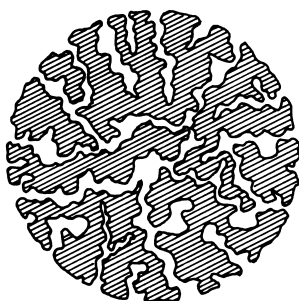
Fig. 2.5 Pore structure of a stationary phase particle.
