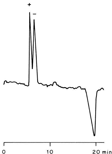
Figure 21.2 Separation of N -(1-phenylethyl)phthalamic acid enantiomers with a chiral ion-pair reagent. (Reproduced with permission from C. Pettersson, J. Chromatogr. , 316 , 553 (1984).) Conditions: stationary phase, LiChrosorb SI 100, 5 \mu\text{m} ; mobile phase, dichloromethane–butane-1,2-diol (99:1) containing 0.35 mM each of quinine and acetic acid; UV detector. The negative peak at ca. 19 min is a system peak.
