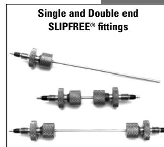
The locking nut allows the SLIPFREE tubing to extend into the fitting to ensure a zero dead volume seal in all column fittings.
