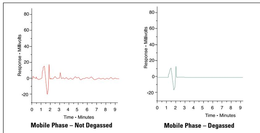
The most efficient form of degassing is bubbling with helium or another low solubility gas. If this method is available, we recommend that the mobile phase is continually degassed at very low levels throughout the analysis. This will inhibit the re-adsorption of gases over the analysis time.
