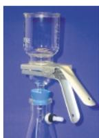
Ideally, all HPLC solvents should be filtered through a 0.45  $\mu\text{m}$  filter before use. This removes any particulate matter that may cause blockages. After filtration, the solvents should be stored in a covered reservoir to prevent contamination with dust etc. Filtering HPLC solvents will benefit both your chromatography and the wear and tear of the HPLC system. Pump plungers, seals and check valves will perform better and lifetimes will be maximized.
