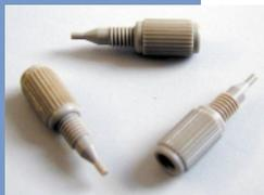
These units are positioned between the solvent inlet filter and the column inlet. They are designed to trap particulates from the fluid path. They will not trap dissolved substances. Once again, these units are designed to be disposable and should be replaced regularly. There are a number of designs of filters available. For further information on these designs or for advice on your application, please contact your Thermo representative.
