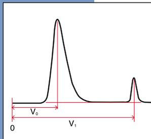
**Important:** The column void volume can be measured by injecting a compound that will be unretained by the column packing. Typical compounds used include uracil (RP) and toluene (NP). Contact your column supplier for advice if you are unsure about the retention characteristics of your chosen void marker.
