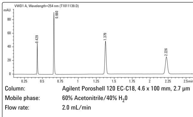
Figure 1. Agilent Poroshell 120 EC-C18 chromatogram.
