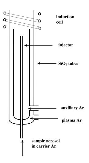
The torch consists of three concentric quartz tubes (the injector tube is made of quartz or corundum or sapphire) positioned co-axially in an induction coil (made of copper). Argon flows through the individual tubes.
