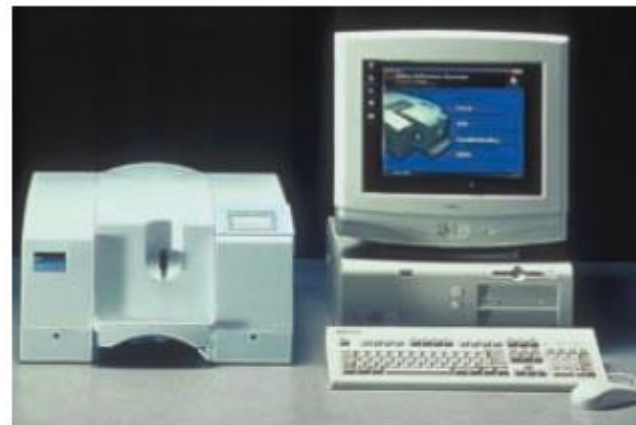
FIGURE 7 The infrared spectrophotometer shown here produces a chemical fingerprint of a substance.
