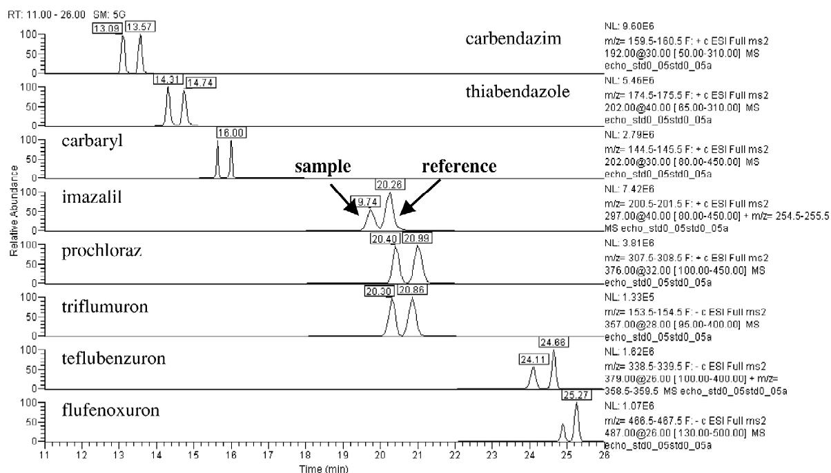
Fig. 3. LC–MS chromatogram of pesticide mixture—application of echo-peak injection 10  $\mu$ l injection. 1st peak, sample: standard of pesticides (0.5  $\mu$ g/ml) in methanol–water (1:1, v/v). 2nd peak, reference: standard of pesticides (0.5  $\mu$ g/ml) in methanol–water (1:1, v/v).
