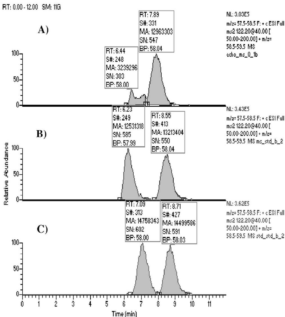
Fig. 5. Chromatograms of chlormequat obtained by echo-peak technique; (A) injection 1, standard (0.1  $\mu\text{g/ml}$ ); injection 2, sample of pear concentrate (0.1  $\mu\text{g/ml}$ ). (B) Injection 1, sample of pear concentrate (0.1  $\mu\text{g/ml}$ ); injection 2, standard (0.1  $\mu\text{g/ml}$ ). (C) Injection 1, standard (0.1  $\mu\text{g/ml}$ ); injection 2, standard (0.1  $\mu\text{g/ml}$ ).
