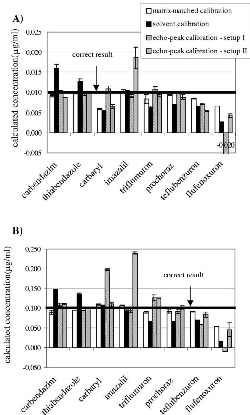
Fig. 4. Accuracy of data obtained by different calibration techniques, GPC purified apple extracts (1 g/ml) spiked with pesticides (mixture A): (A) sample at 0.01  $\mu\text{g/ml}$ ; (B) sample at 0.1  $\mu\text{g/ml}$ .
