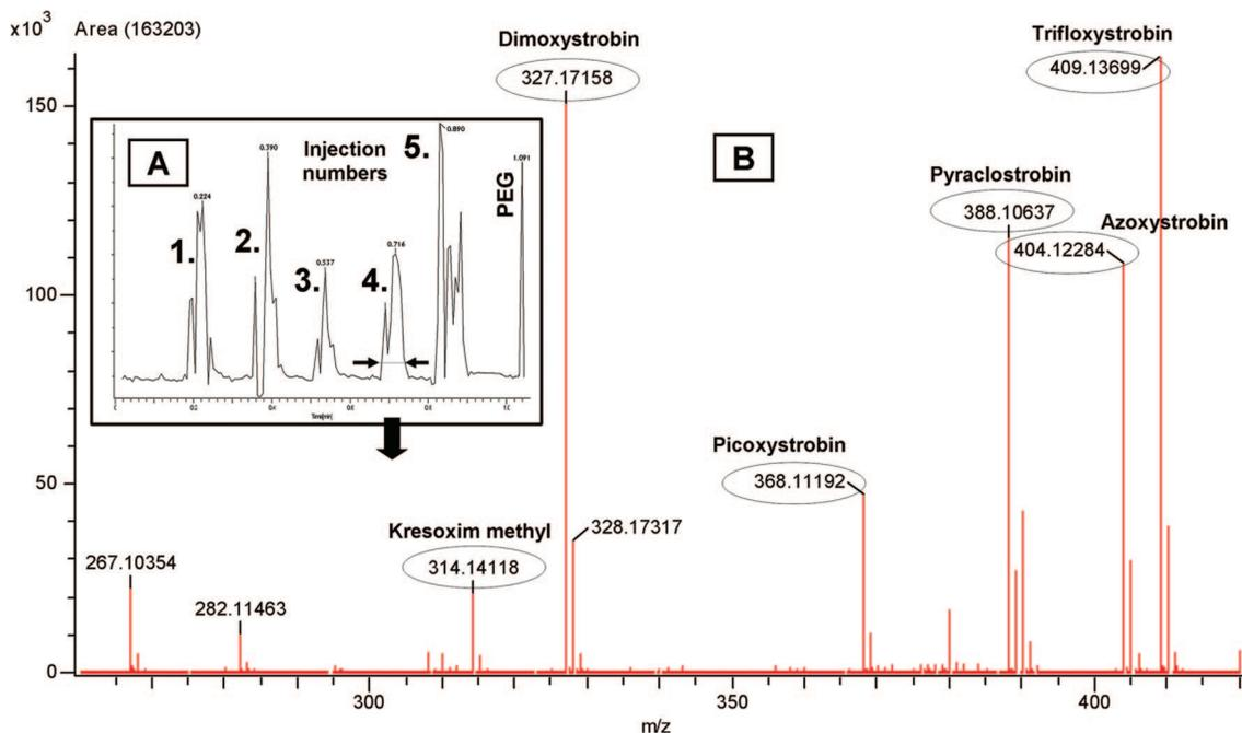
**Figure 1.** DART-TOF MS analysis of crude ethyl acetate extract of wheat grains spiked with strobilurins at  $50 \mu\text{g kg}^{-1}$ . (A) Total ion current (five repeated injections plus PEG 600). (B) Zoomed part of  $[M + H]^+$  mass profile in the  $m/z$  range 310–410 (example for injection four).
