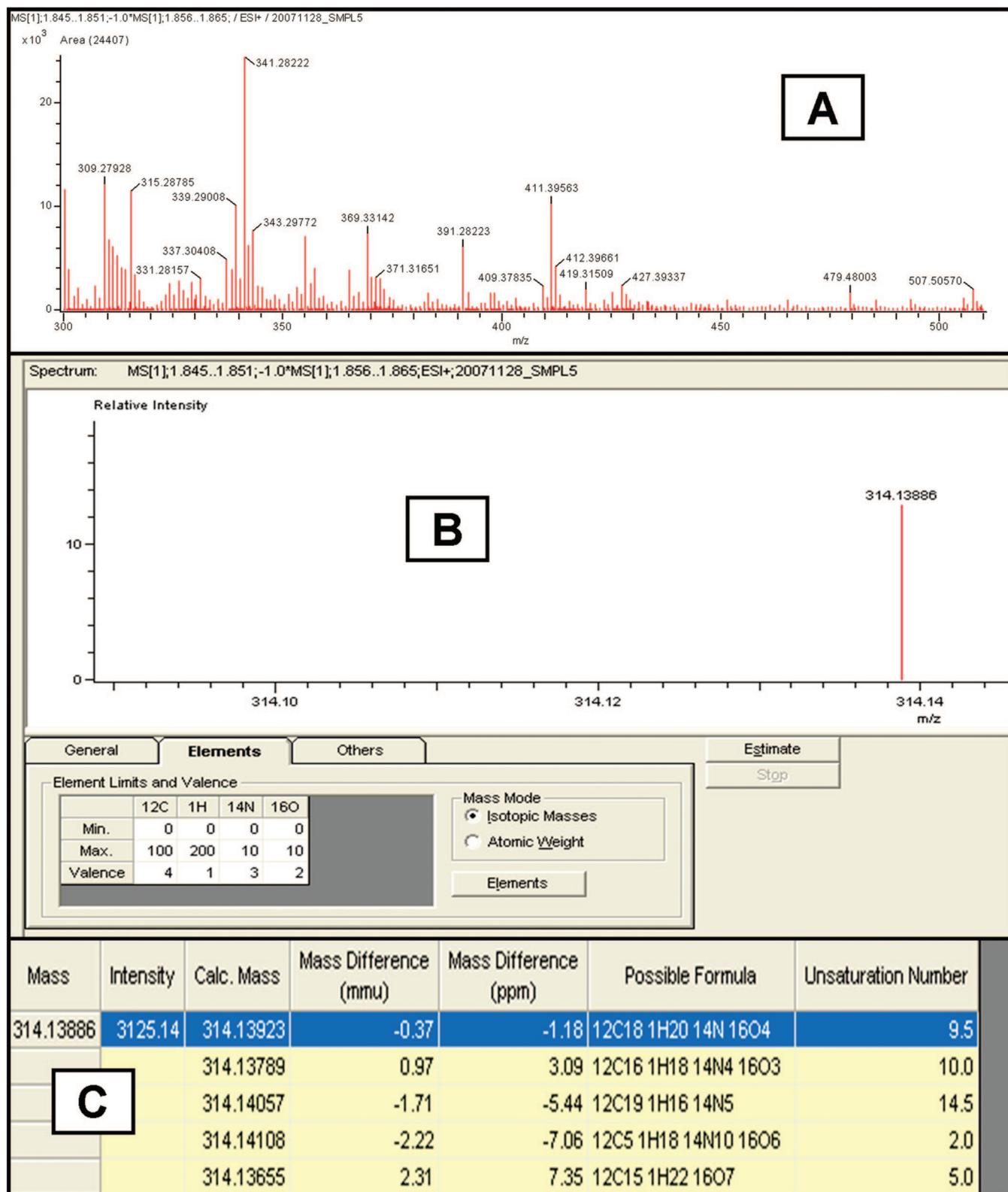
**Figure 2.** DART-TOF MS direct analysis of wheat grains, element composition report. (A) Mass profile of the BIOCOP test sample with incurred kresoxim-methyl. (B) Zoomed part of mass profile showing in particular  $[M + H]^+$  of kresoxim-methyl. (C) Estimating elemental composition from accurate mass measurement, the highlighted column stands for target analyte.
