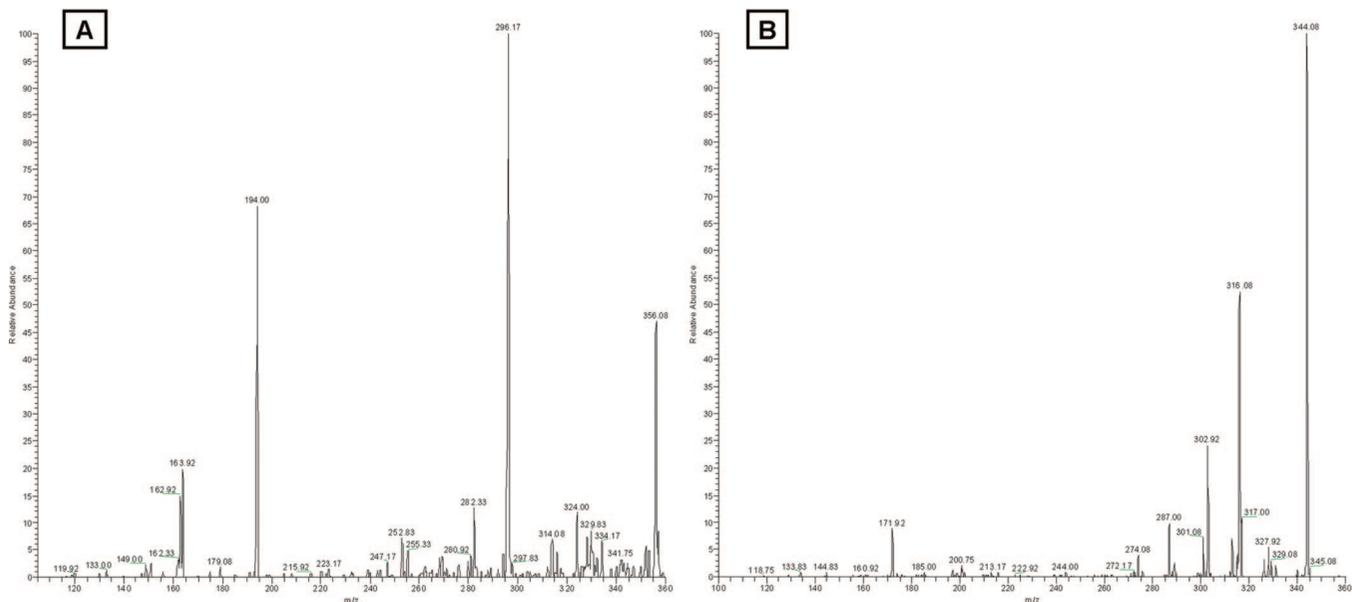
**Figure 3.** DESI-LIT MS<sup>n</sup> confirmatory analysis of wheat samples incurred with strobilurin fungicides. (A) MS<sup>2</sup> full scan product ion spectrum of pyraclostrobin (*m/z* 388). (B) MS<sup>3</sup> full scan product ion spectrum of azoxystrobin (*m/z* 404 → 372). The concentrations as determined by LC–MS/MS are given in Table 5.
