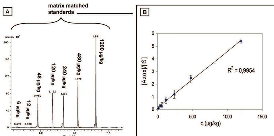
**Figure 4.** Quantification using DART-TOF MS. (A) Single ion current of *m/z* 404.1246 (azoxystrobin [M + H]<sup>+</sup> value) in matrix matched calibration standards (6–1200 µg kg<sup>-1</sup>) measured within a single run. (B) Working curve of azoxystrobin (analyte to internal standard intensity ratio plotted versus analyte concentration).
