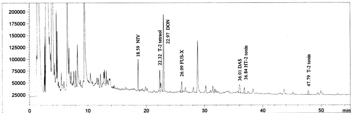
Fig. 6. Chromatogram of spiked rice sample (0.3 mg/kg); clean-up on a MycoSep 225 column; injection corresponds to 43.2 pg of each toxin in 0.144 mg sample. Axes as in Fig. 3.
