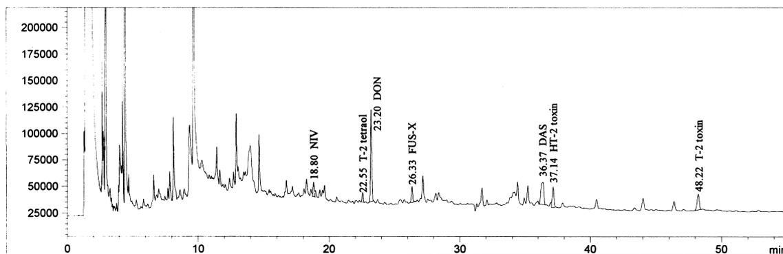
Fig. 4. Chromatogram of spiked wheat sample (0.5 mg/kg); clean-up on Florisil+C<sub>18</sub>-silica gel cartridges; injection corresponds to 180 pg of each toxin in 0.36 mg sample. Axes as in Fig. 3.
