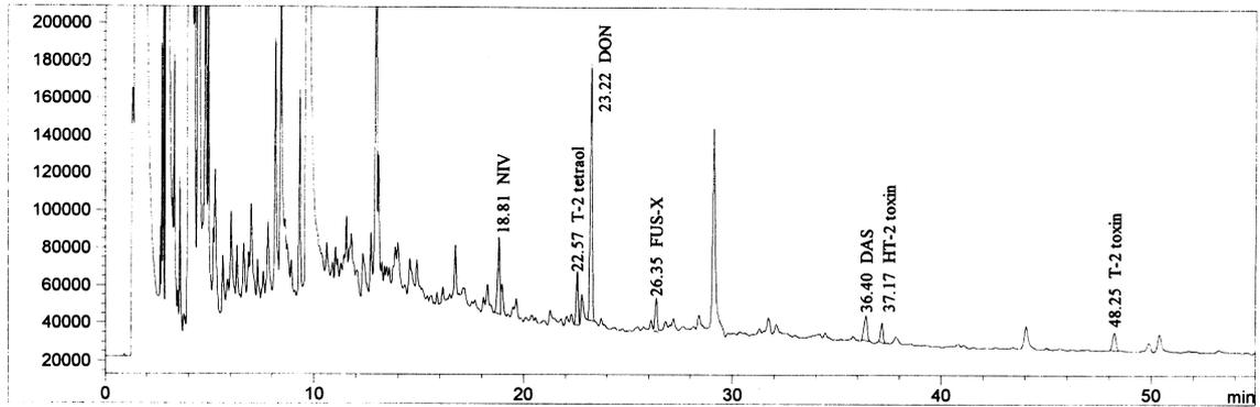
Fig. 5. Chromatogram of spiked wheat sample (0.5 mg/kg); clean-up on a MycoSep 225 column; injection corresponds to 72 pg of each toxin in 0.144 mg sample. Axes as in Fig. 3.
