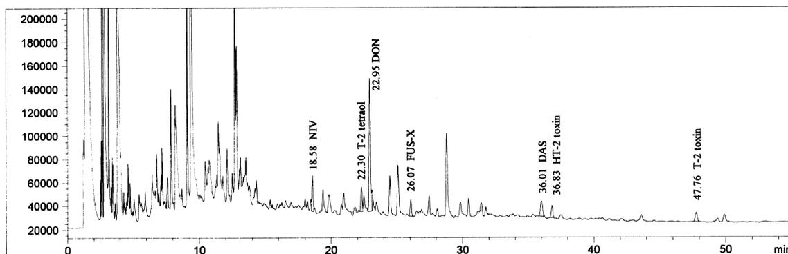
Fig. 7. Chromatogram of spiked corn sample (0.3 mg/kg); clean-up on a MycoSep 225 column; injection corresponds to 43.2 pg of each toxin in 0.144 mg sample. Axes as in Fig. 3.
