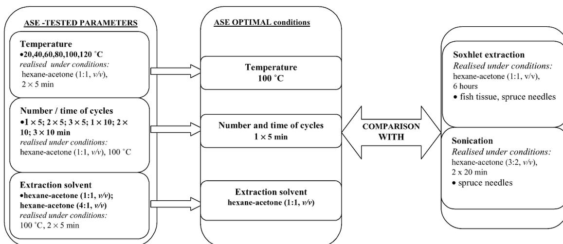
Fig. 1. Overview of testing of the PLE performance: experimental set-up.
