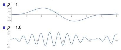
When *p* approaches  $\omega$ , the maximal amplitude grows.
