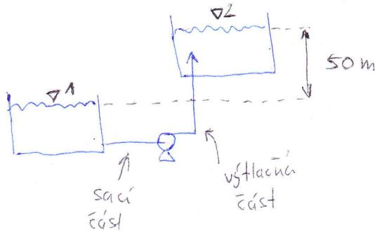
nové ocelové  $\epsilon_A = 0.2 \text{ mm}$  $d = 0.1 \text{ m}$  $e_{dis, sací} = 15.3 \text{ J/kg}$  $L = 400 \text{ m}$  $\xi_f = 9.2$  $V = 1.3 \text{ m/s}$  $\gamma_{cell} = 0.76, P = ?, \dot{V} = ?$
