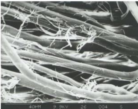
Figure 4. Enzymatic treatment on jet, AIRO 1000 and dried on AIRO
