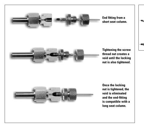
The locking nut allows the SLIPFREE tubing to extend into the fitting to ensure a zero dead volume seal in all column fittings.
