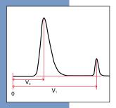
Capacity factor is a measure of the retention of an analyte relative to the column void volume,  $V_0$ . It is measured using the following equation:
